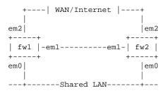
The firewalls are connected back-to-back using a crossover cable on em1. Both are connected to the LAN on em0 and to a WAN/Internet connection on em2. IP addresses are as follows:
